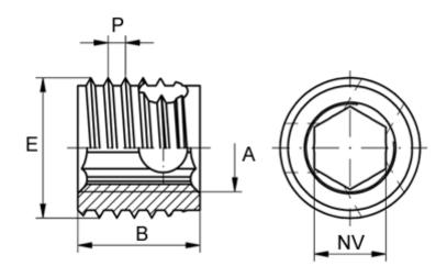
Female thread A = M10= 18 Length B Male thread E = 14 Min hole depth blind hole = 22 Min material thickness = 18 = -SW Thread pitch P = 1.5
